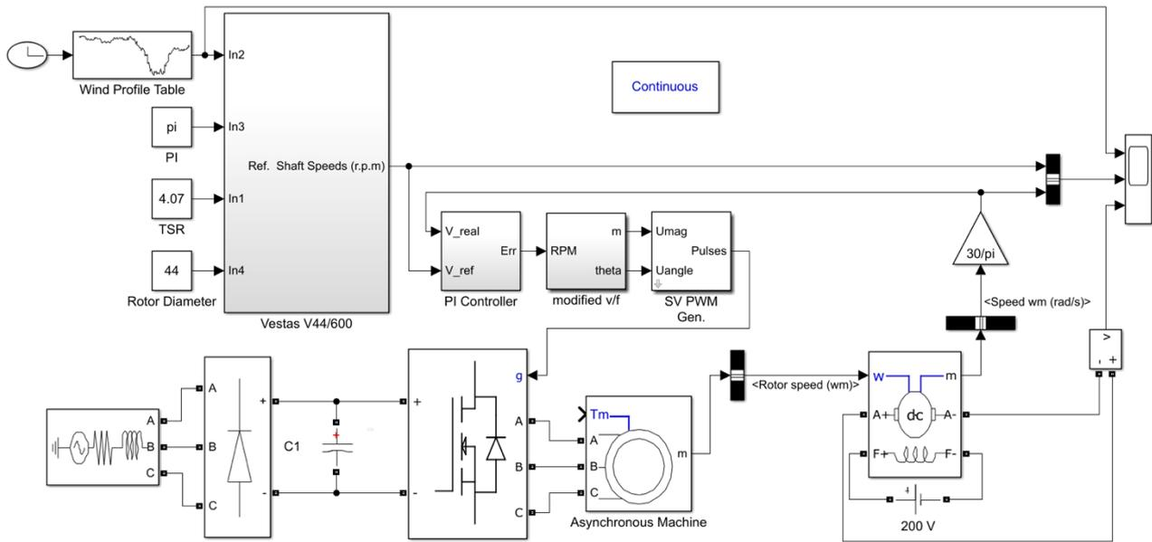
**Fig. 1.** Simulink model of the proposed WTE.
