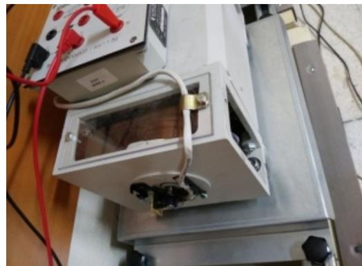
Fig. 11. Optical incremental encoder designed to read motor shaft speed.
