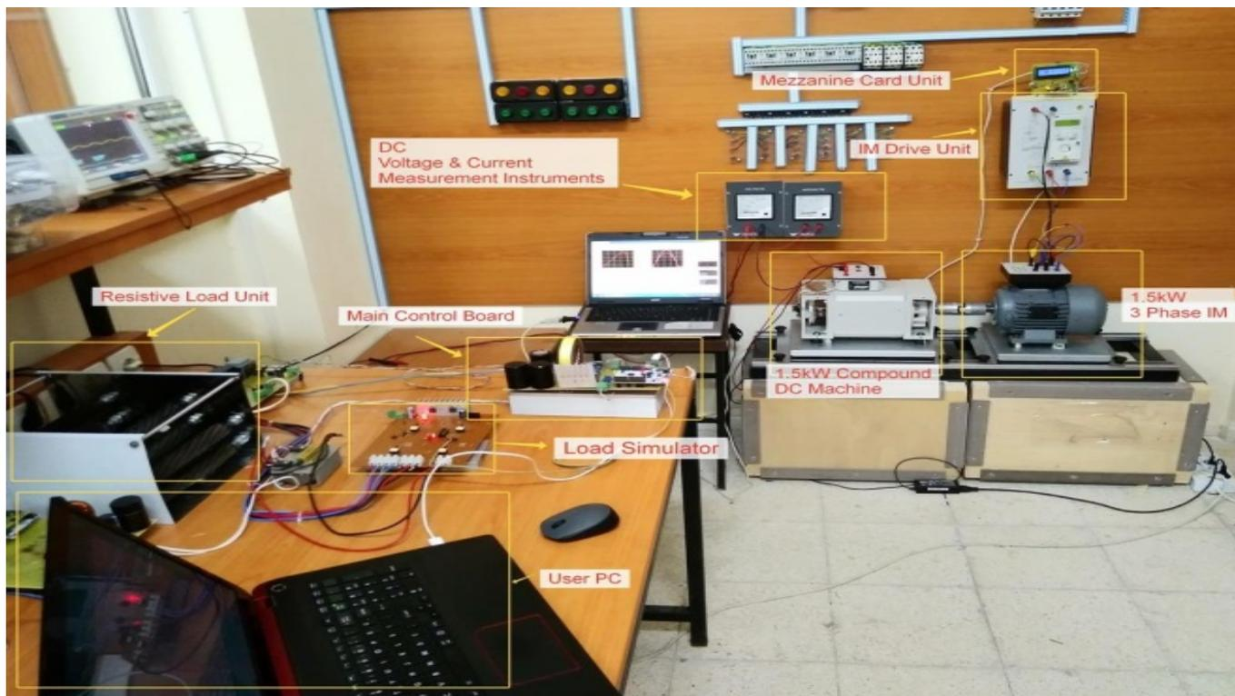
Fig. 18. The experimental setup of the designed WTE system and its components.
