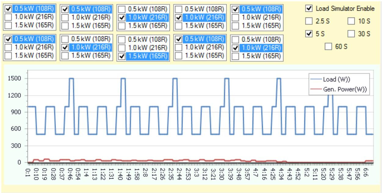
Fig. 6. Load simulator control stage in user interface.
