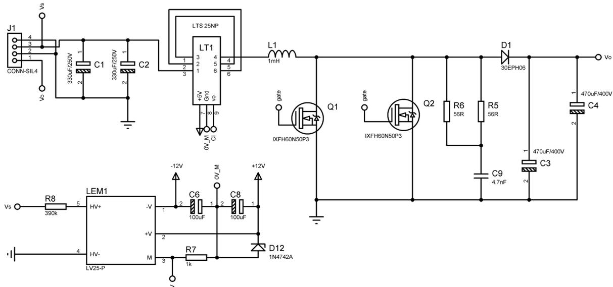
**Fig. 13.** The electronic circuit diagram of the power stage of the designed converter.
