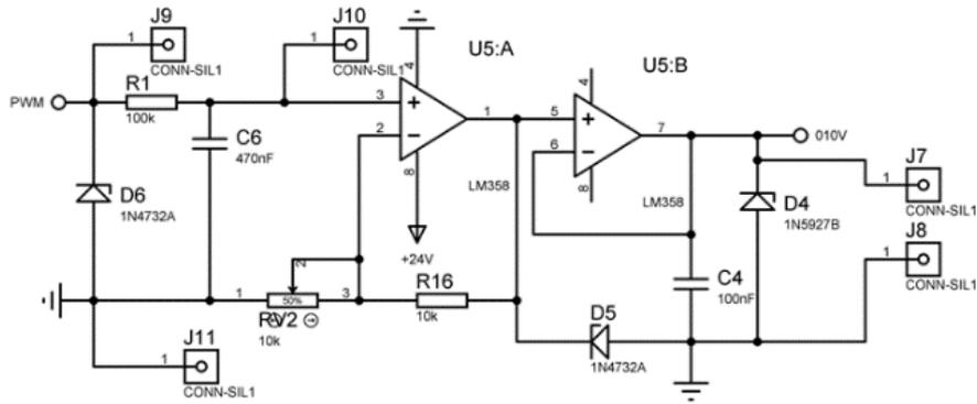
Fig. 9. 4-20mA signal generator circuit for motor driver unit.
