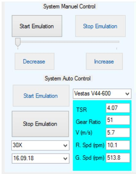
Fig. 5. Wind turbine, date selection and control options.
