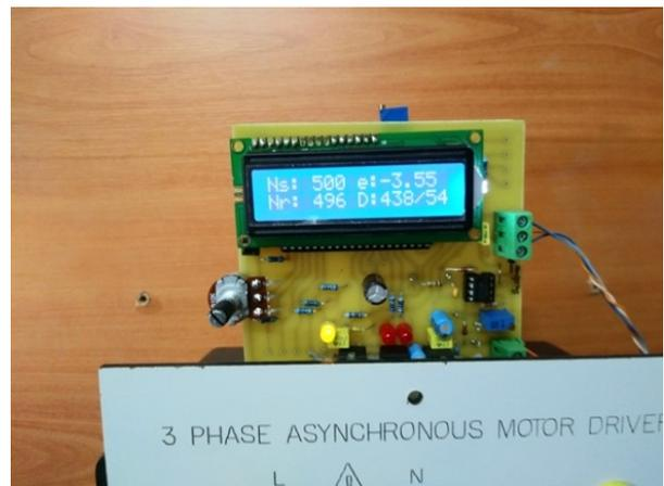
Fig. 8. The mezzanine board unit that controls the drive and the components of the board.
