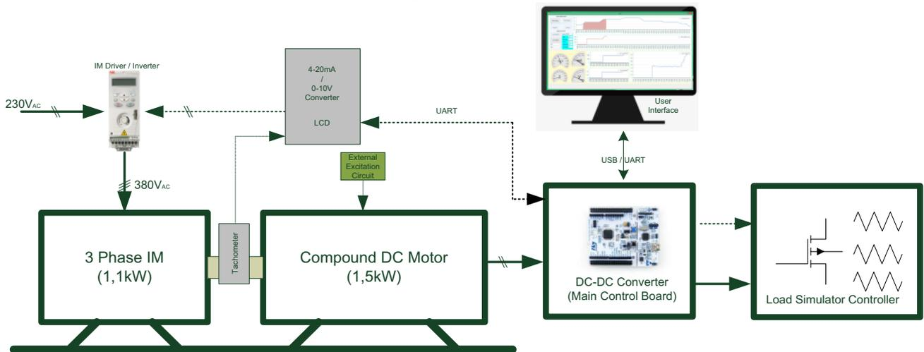
Fig. 3. The proposed WTE configuration.
