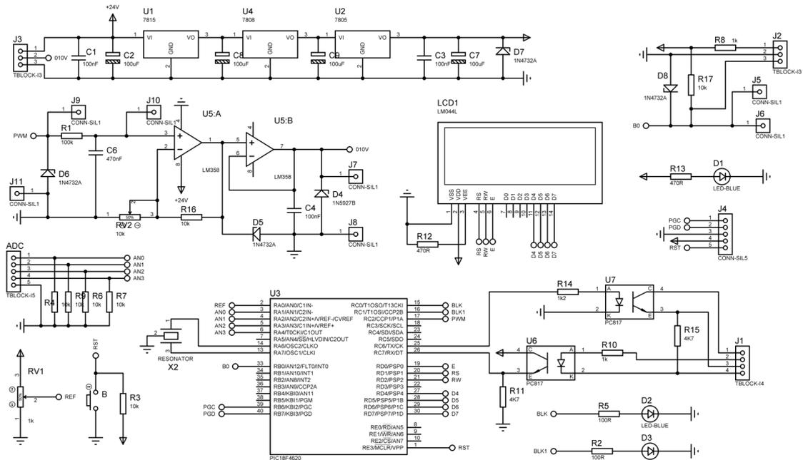
Fig. 10. The mezzanine board unit that controls the drive and the components of the board.
