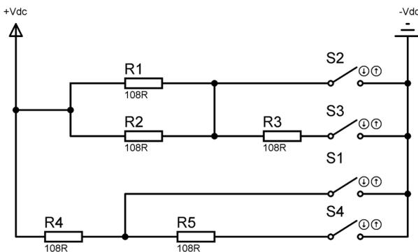
Fig. 7. Connection diagram of loads.
