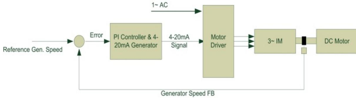
**Fig. 12.** The mezzanine board and motor driver for WTE.
