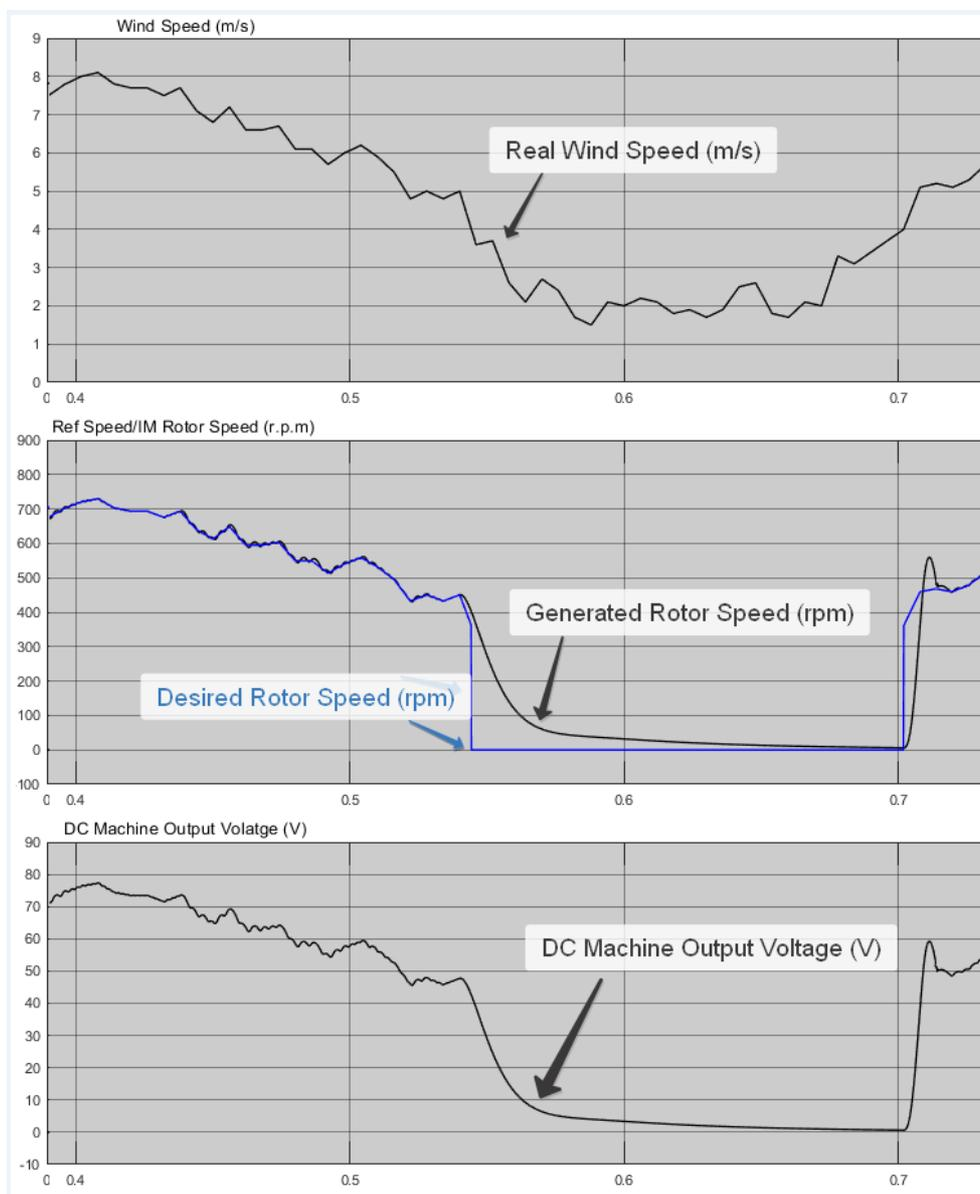
**Fig. 17.** Real wind speed, generated rotor speed, and DC machine output voltage characteristics demonstrating the cut-out of the system below 4 m/s.
