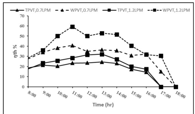
Fig.14. The hourly variation of average thermal efficiency vs. time for both hybrid collectors in March.
