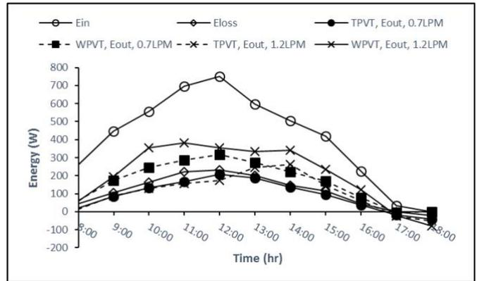
Fig.9. Average energy vs time simulation for both hybrid PVT collectors.in February.
