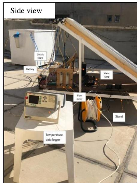
**Fig. 2.** Photograph of the experimental device
