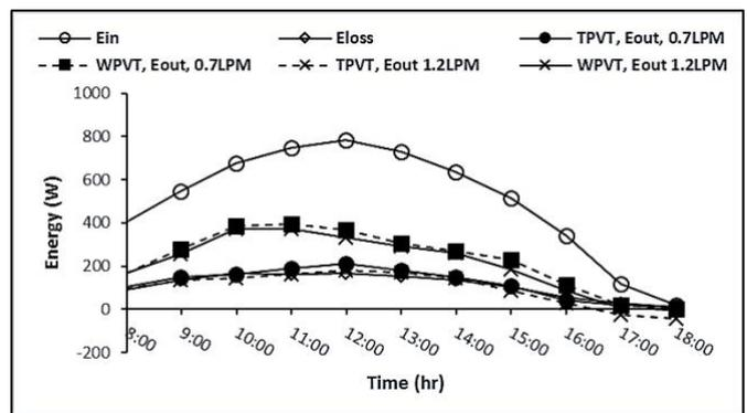
Fig.11. Average energy vs time simulation for both hybrid PVT collectors.in April.
