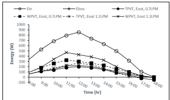
Fig.10. Average energy vs time simulation for both hybrid PVT collectors.in March.
