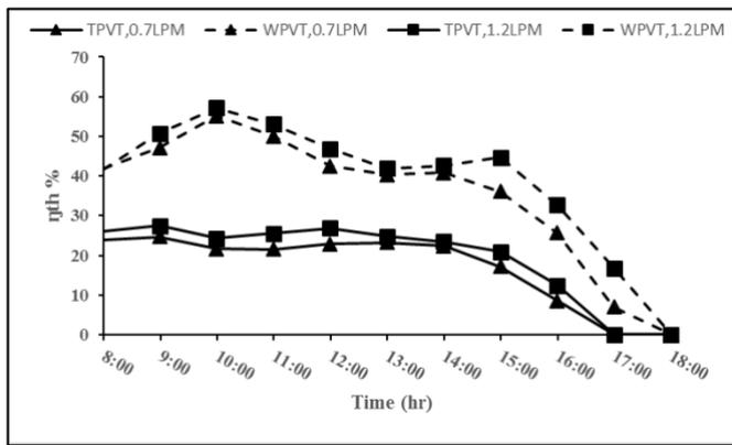
**Fig.15.**The hourly variation of average thermal efficiency vs. time for both hybrid collectors in April.
