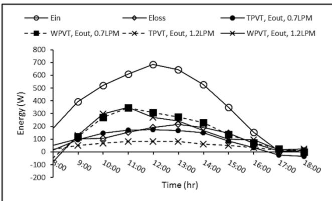
Fig.8. Average energy vs time simulation for both hybrid PVT collectors.in January.
