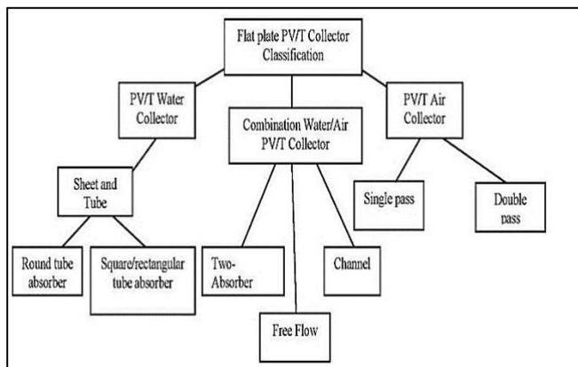
**Fig. 1.** Flat plate PVT collector classification [12].
