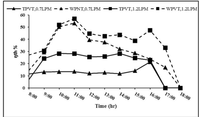
Fig.12. The hourly variation of average thermal efficiency vs. time for both hybrid collectors in January.
