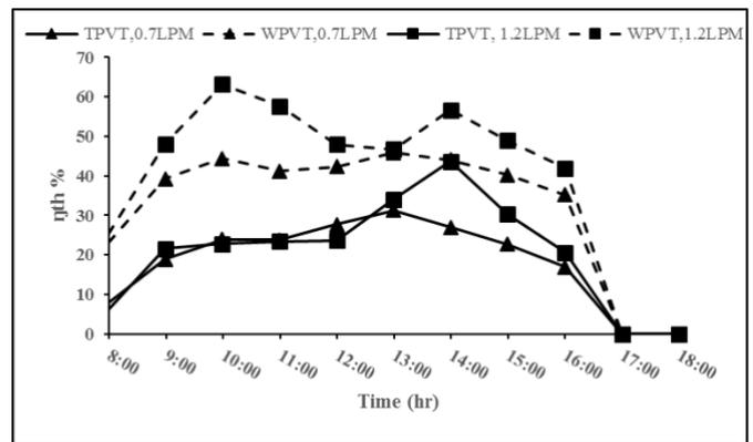
Fig.13. The hourly variation of average thermal efficiency vs. time for both hybrid collectors in February.
