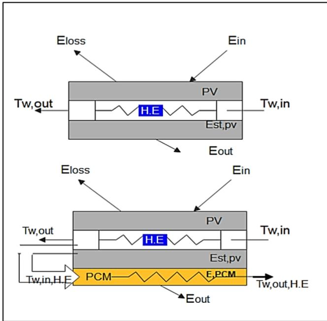
Fig. 3. The system’s energy balance process
