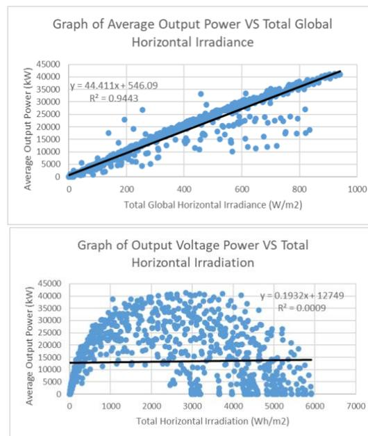
**Fig. 3.** Graph of Average Output Power vs Total Global Horizontal Irradiance and total horizontal irradiation before Filtration
