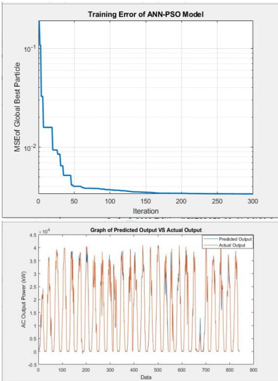
**Fig. 13.** Training Performance of ANN-PSO Model and Predicted Output Vs Actual Output of AC Output Power
