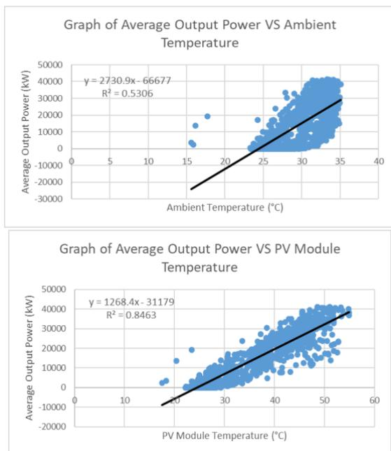
**Fig. 5.** Graph of Average Output Power vs Ambient Temperature before filtration and PV module temperature before Filtration
