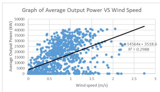
**Fig. 6.** Graph of Average Output Power vs Wind Speed before Filtration
