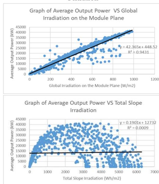
**Fig. 4.** Graph of Average Output Power vs Global Irradiance on The Module Plane and Total Slope Irradiation before Filtration
