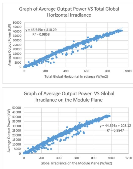
**Fig.7.** Graph of Average Output Power vs Total Global Horizontal Irradiance and Global Irradiance on the Module Plane after Filtration
