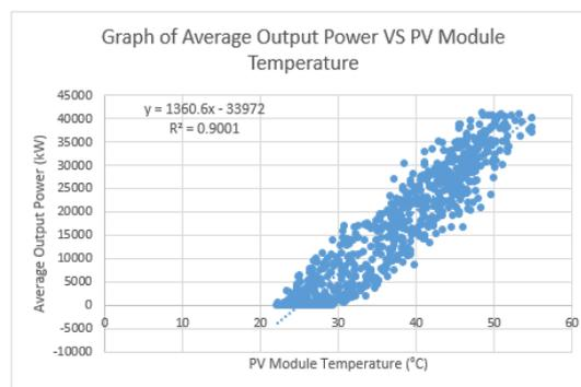
**Fig. 8.** Graph of Average Output Power vs PV Module Temperature after Filtration
