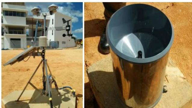
**Fig. 2.** Weather station located at Gambang LSS Farm (left) and tipping bucket rain gauge (right)
