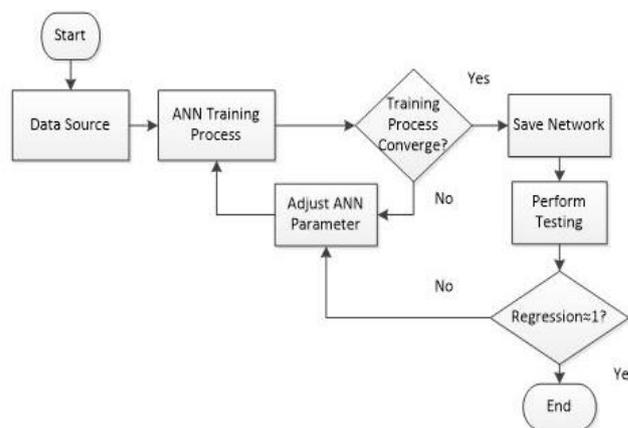
**Fig. 10.** Flowchart for ANN training and testing process
