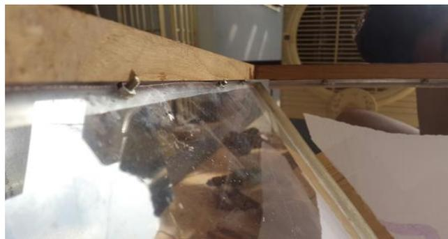
**Fig. 7.** Wooden frame and Al-bends bolted to fiber glass
