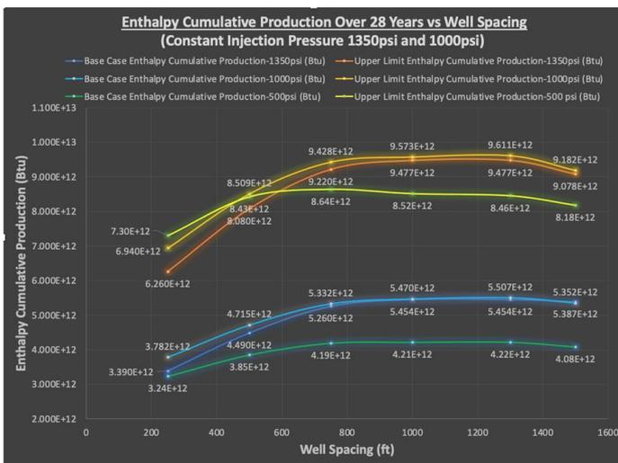
Fig. 16. Enthalpy Cumulative Production at Various Well Spacings for a 28-year period for Base and Upper Limit Case at Constant Injection Pressures of 1350psi, 1000psi and 500psi
