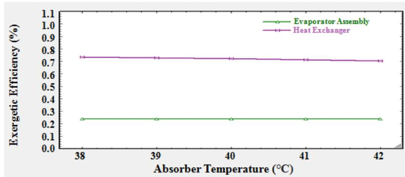
Fig. 5. Variation of exergetic efficiency of the components for different absorber temperatures [44]
