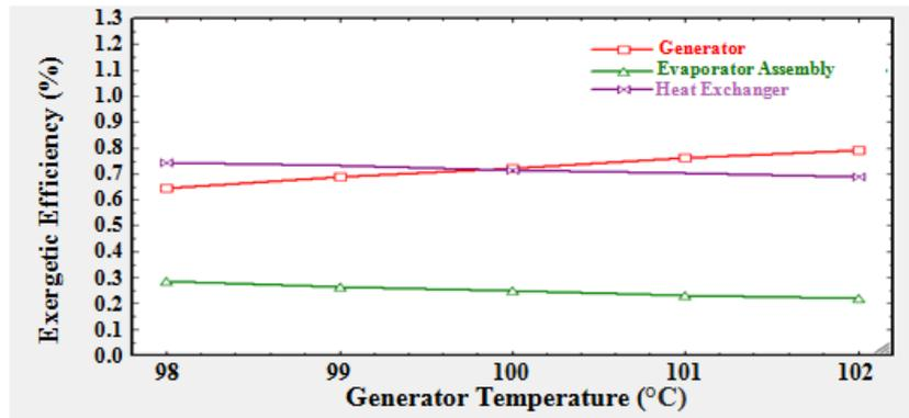
**Fig. 4.** Variation of exergetic efficiency of the components for different generator temperatures [44]
