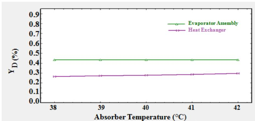
Fig. 7. Variation of  $Y_D$  of the components for different absorber temperatures [44]
