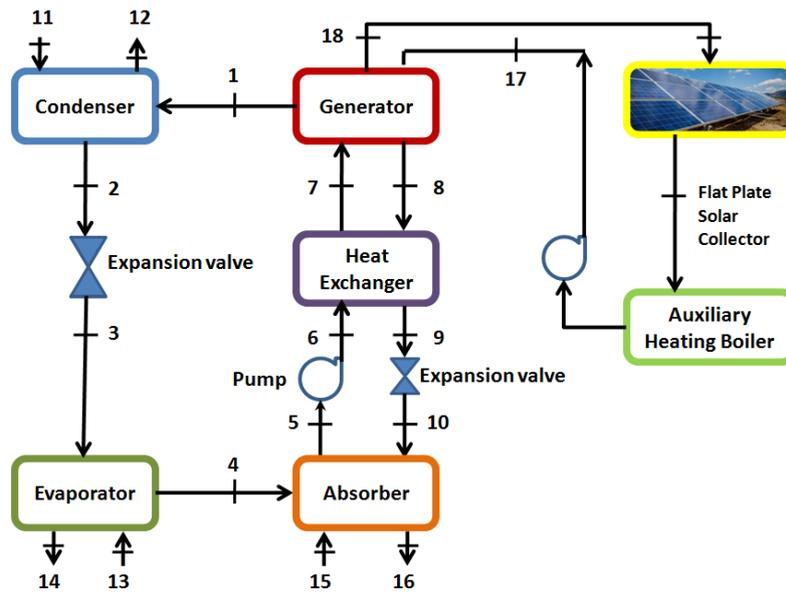
Fig. 1. Solar assisted absorption cooling system scheme[43]
