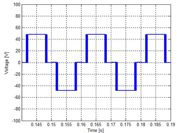
**Fig. 5.** Simulation result of the output voltage of the four-wire inverter that connects to terminal b and single-phase inverter connecting terminal a.
