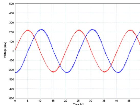
**Fig. 15.** Experimental result of the output currents  $I_a$  and  $I_c$  of the multilevel inverter (100mV - 1A).
