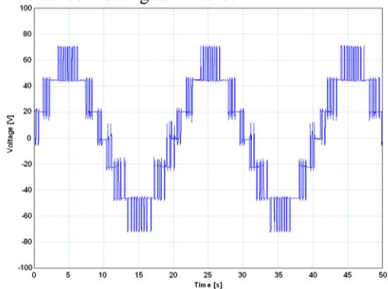
**Fig. 13.** Experimental result of the output voltage  $V_{ab}$  of the multilevel inverter.
