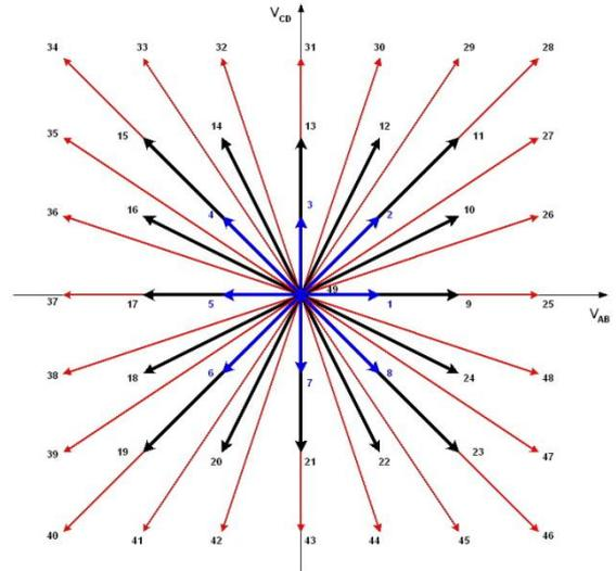
**Fig. 4.** Output voltage vectors of the proposed multilevel inverter.
