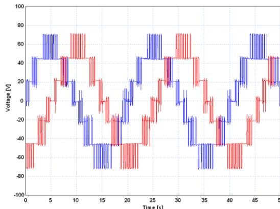
**Fig. 14.** Experimental result of the output voltages  $V_{ab}$  and  $V_{cd}$  of the multilevel inverter.
