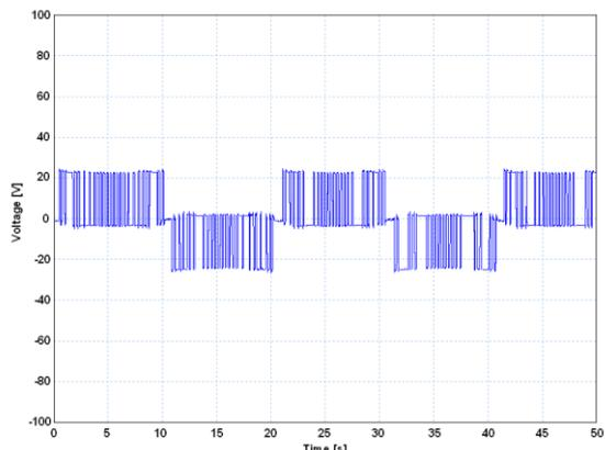
**Fig. 12.** Experimental result of the output voltage of the single-phase inverter that connects to terminal a and four-wire inverter connecting terminal b.
