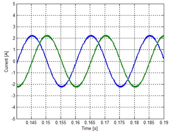
**Fig. 9.** Simulation result of the output currents  $I_a$  and  $I_c$  of the multilevel inverter.
