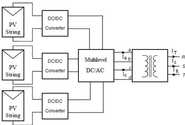
**Fig. 1.** Configuration of the proposed grid connected photovoltaic system.
