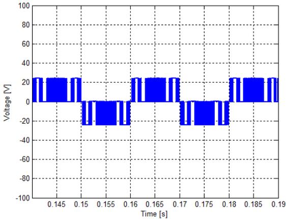
**Fig. 6.** Simulation result of the output voltage of the single-phase inverter that connects to terminal a and four-wire inverter connecting terminal b.
