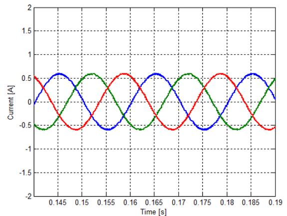
**Fig. 10.** Simulation result of the output currents  $I_R$ ,  $I_S$  and  $I_T$  of the Le-Blanc transformer.
