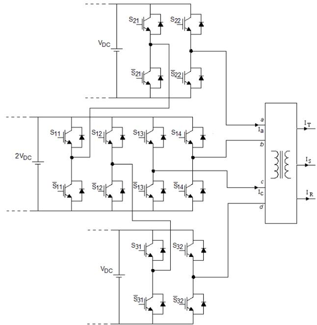
**Fig. 2.** Multilevel DC/AC converter.
