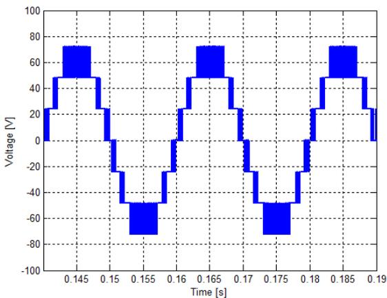
**Fig. 7.** Simulation result of the output voltage  $V_{ab}$  of the multilevel inverter.
