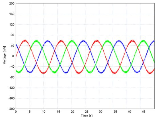
**Fig. 16.** Experimental result of the output currents  $I_R$ ,  $I_S$  and  $I_T$  of the Le-Blanc transformer (100mV - 1A).
