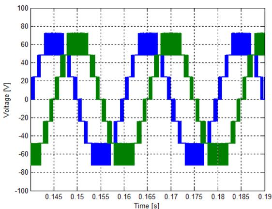
**Fig. 8.** Simulation result of the output voltages  $V_{ab}$  and  $V_{cd}$  of the multilevel inverter.
