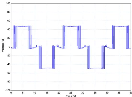
**Fig. 11.** Experimental result of the output voltage of the four-wire inverter that connects to terminal b and single-phase inverter connecting terminal a.
