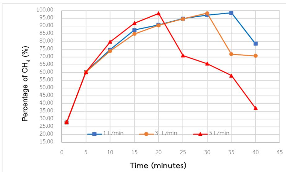
**Fig 3.** The influences of feed flow rates on the CH<sub>4</sub> purity
