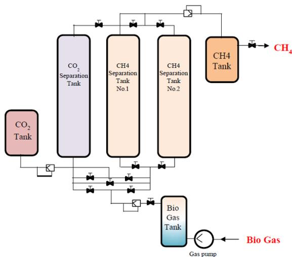
(a) Biogas separation system
