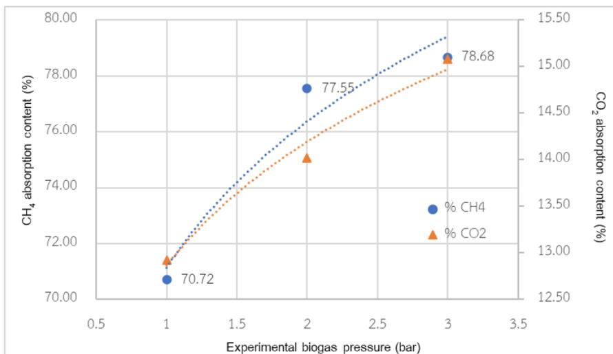
**Fig 2.** Comparison of methane and carbon dioxide adsorption at different pressure
