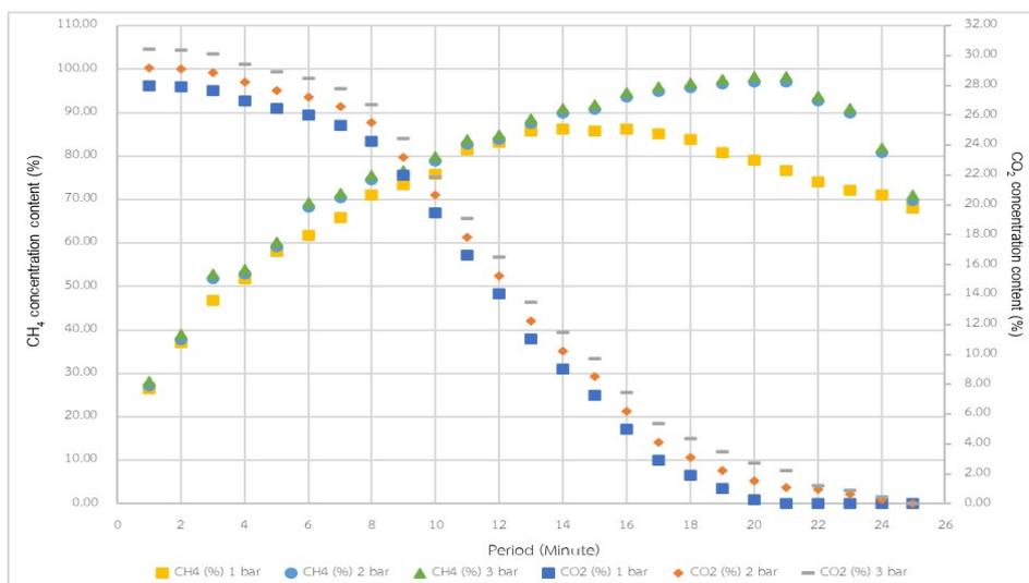
Fig 4. The concentrations of CH<sub>4</sub> (left side) and CO<sub>2</sub> (right side) of biogas at different total pressures
