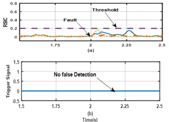
**Fig.7.** (a) RSIC for the short circuit faults (b) Trigger signal.
