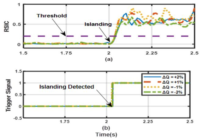
**Fig.6.** (a) RSIC for the impact of varying reactive power (b) Trigger signal.
