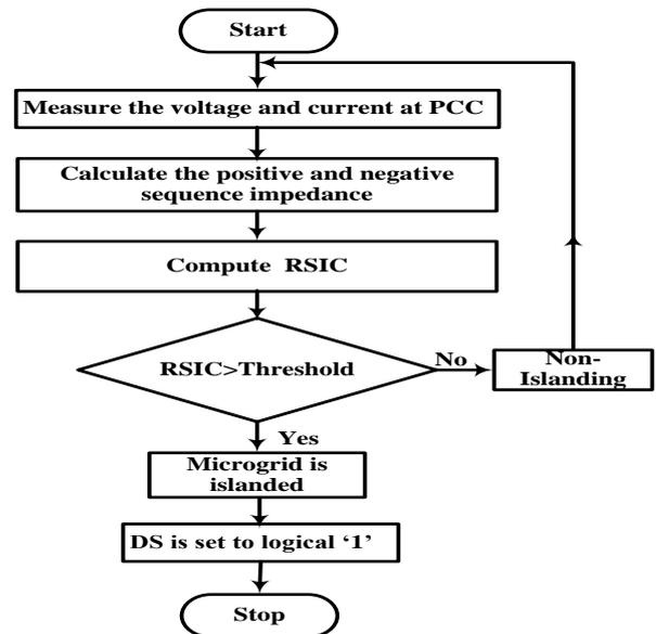
Fig. 2. Flow chart for the proposed detection technique.
