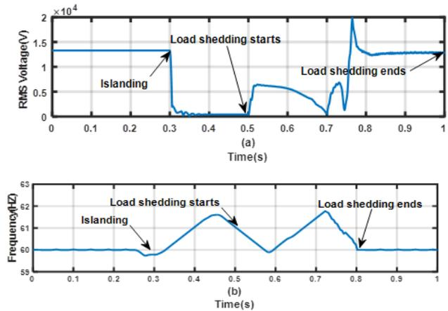
Fig.10. (a) RMS voltage (b) Frequency for load shedding.
