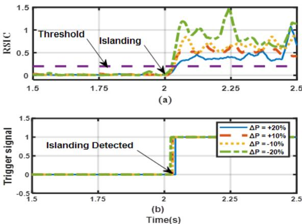
**Fig.5.** (a) RSIC for the impact of varying real power (b) Trigger signal.
