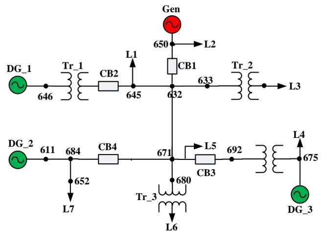
**Fig. 1.** System under consideration for proposed islanding detection technique.
