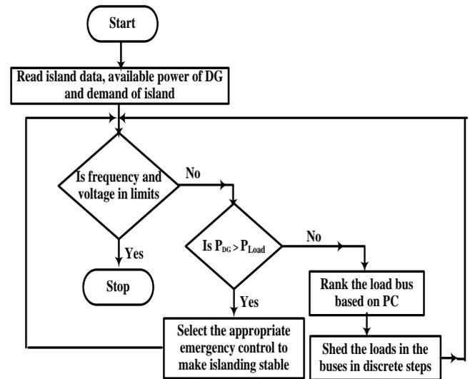
Fig. 3. Flowchart of Proposed Priority Based Load Shedding method.
