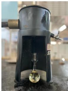
**Fig. 4.** Redwood viscometer to measure viscosity of oil.
