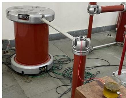
**Fig. 2.** BDV test experimental setup.
