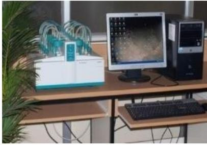
**Fig. 3.** Rancimat 743 test set up to measure oxidation stability.
