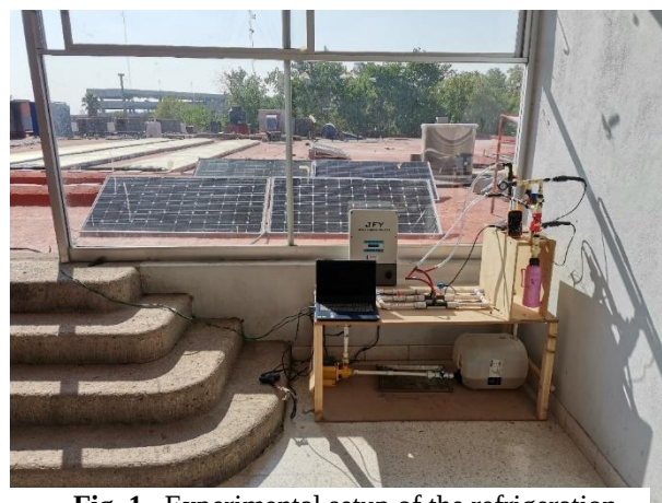
Fig. 1. Experimental setup of the refrigeration device.
