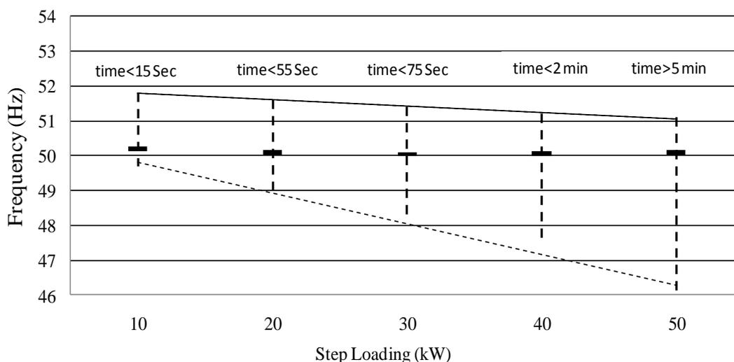
Fig. 4. Fluctuation in frequency of engine gen-set power output by single step loading
