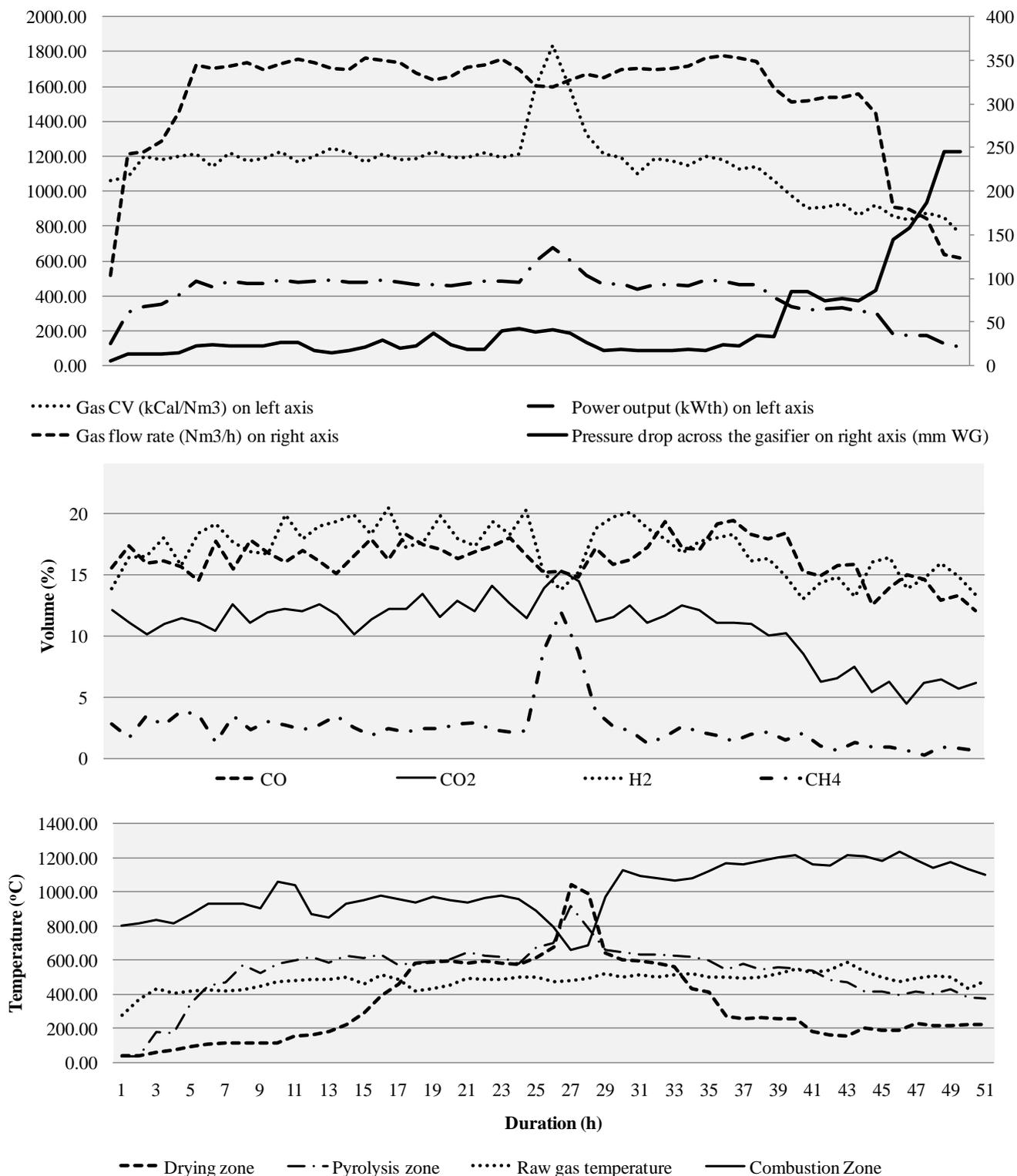
Fig. 2. Overall performance of the gasifier during continuous 50 h operation
