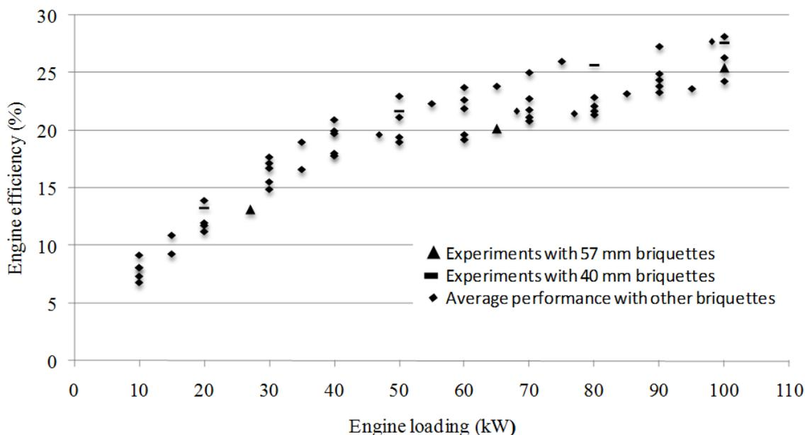
Fig. 3. Efficiency of producer gas based engine gen-set at various loadings
