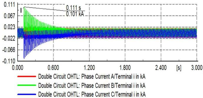
**Fig. 6.** Current flows after single unit transformer energization.
