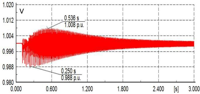
**Fig. 5.** Voltage changes at PCC after single transformer energization.
