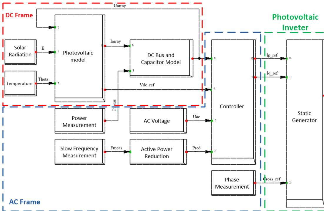
Fig. 2. Composite control farm of the photovoltaic generator.
