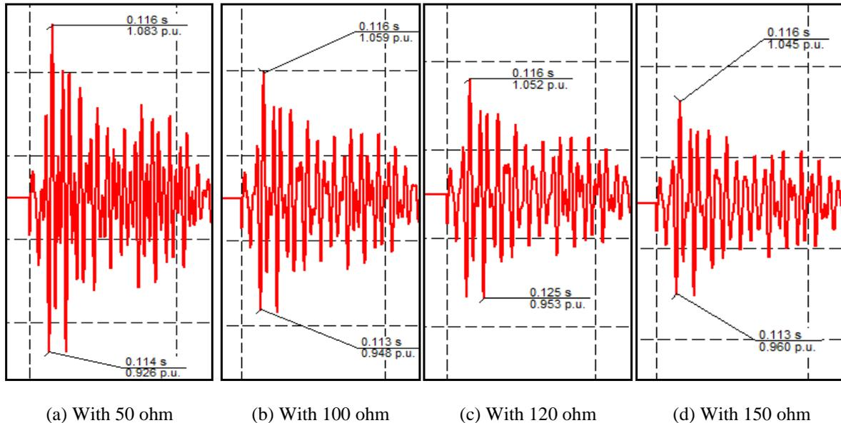
**Fig. 10.** Voltage change at PCC 33kV after the plant energization with different values of Pre-Insertion Resistor; (a) 50 ohm, (b) 100 ohm, (c) 120 ohm, and (d) 150 ohm.
