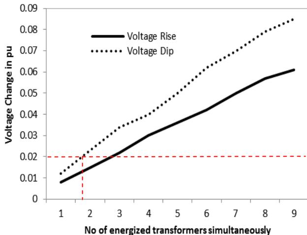
**Fig. 7.** Variation of voltage changes with the number of energized unit transformers.
