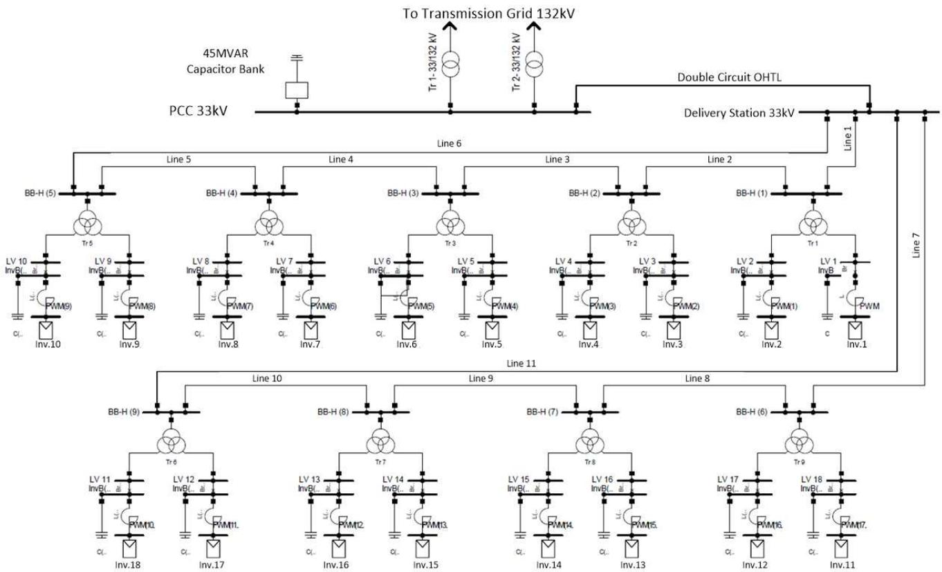
Fig. 1. SLD of the photovoltaic plant implemented by DIgSILENT.
