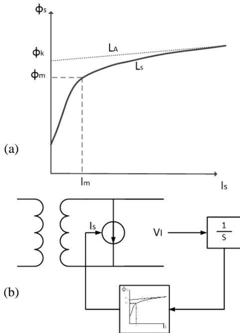
**Fig. 4.** Saturation characteristic of transformers core;
