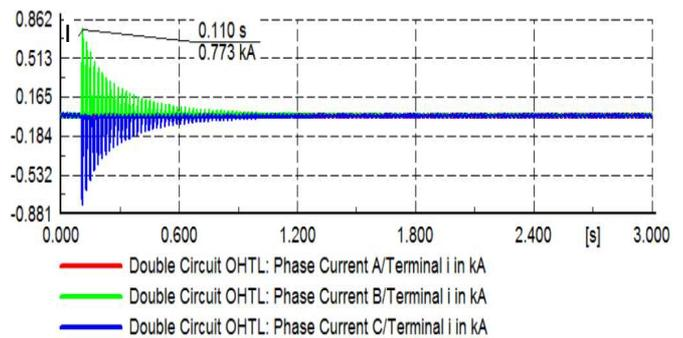
**Fig. 9.** Current flows after the plant energization.
