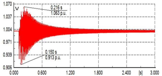
**Fig. 8.** Voltage changes at PCC after plant energization.
