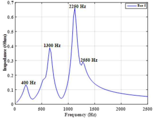
**Fig. 7.** Harmonic resonance at bus 5
