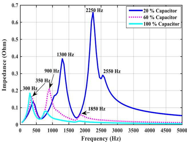
Fig.10. Change in harmonic resonance frequency with variation in capacitor ratings at bus 5
