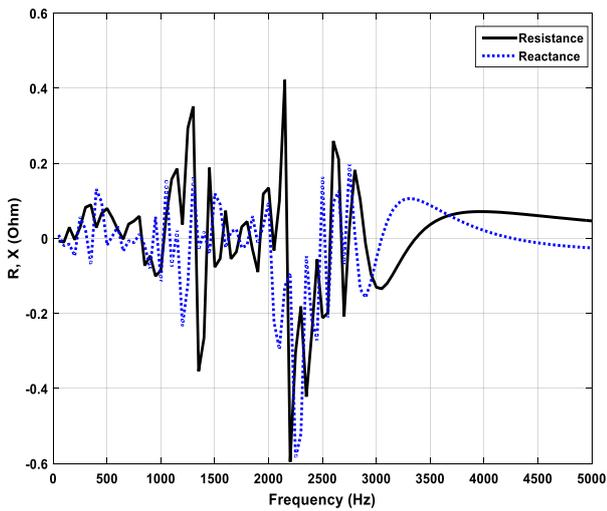
**Fig.6.** Variation in resistance and reactance with frequency at bus 5
