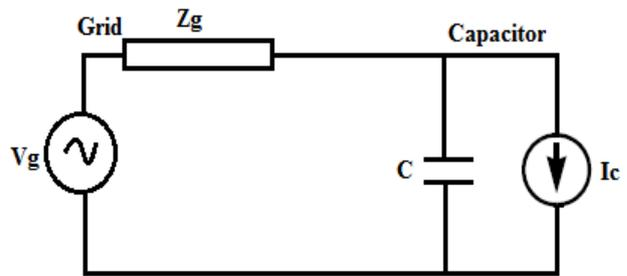
**Fig. 3** Model of capacitor
