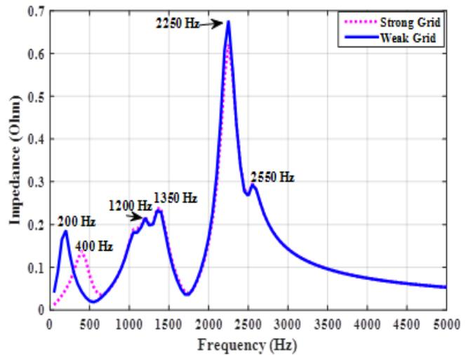
**Fig.8.** Harmonic resonance at bus 5 due to weak and strong grid
