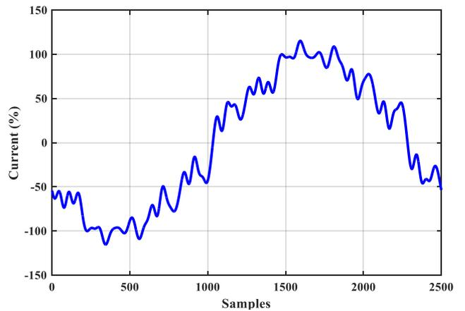
**Fig. 5(b).** Current harmonics waveform between bus 13 & 16
