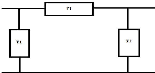
**Fig.2.** Equivalent pi model of cable
