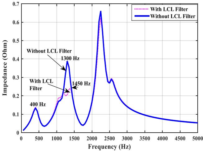
Fig.9. Occurrence of harmonic resonance at bus 5 with and without LCL filter
