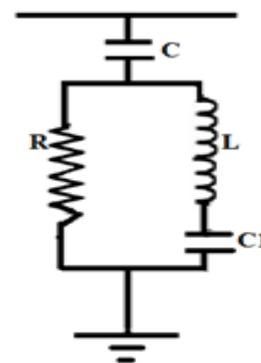
Fig. 12. C-type passive filter
