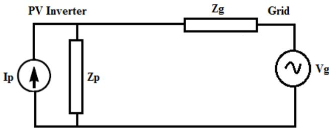
**Fig.1.** Grid inverter model
