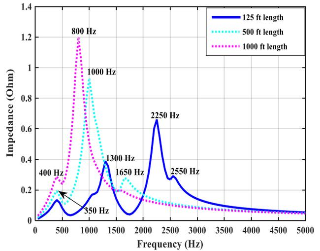
Fig. 11. Change in resonant frequency with cable length
