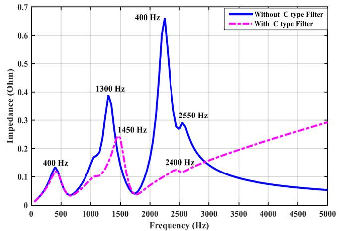
Fig.13. Damping of harmonic resonance frequency with C-type passive filter at bus 5
