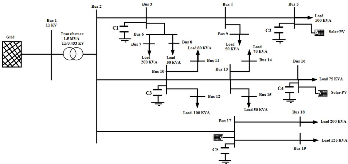
**Fig.4.** Smart rural distribution grid with solar photovoltaic
