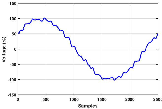
**Fig.4(a).** Voltage harmonics waveform at bus 5
