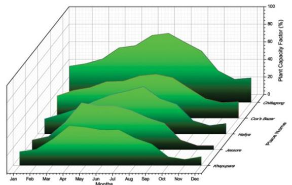
Fig. 23. Average monthly plant capacity factor (PCF) at 120m
