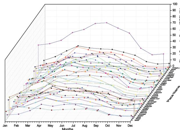
Fig. 18. Average monthly plant capacity factor (PCF) at 50m
