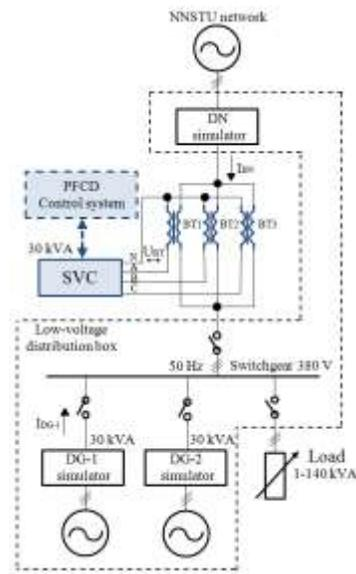
Fig. 6. Physical VPP LV network model scheme with experimental PFCD.
