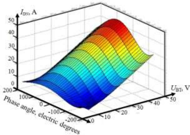
(a) Current in the line DN simulator dependence on output PFCD voltage
