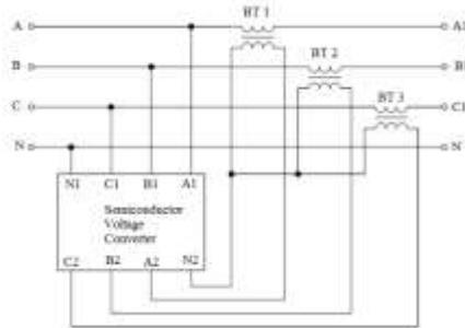
Fig. 4. SVC and booster transformers diagram.
