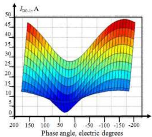
(d) Current amplitude in the line DG-1 simulator dependence on voltage phase angle in the line DN simulator
