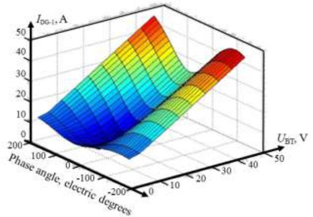
(c) Current in the line DN simulator dependence on output PFCD voltage
