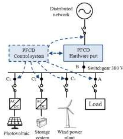
Fig. 5. PFCD application for VPP LV network.
