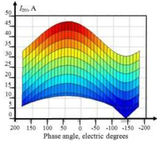
(b) Current amplitude in the line DN simulator dependence on voltage phase angle
