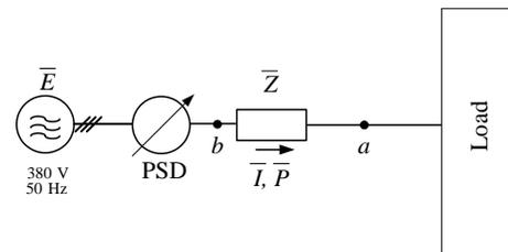
**Fig. 1.** Simplified scheme of power transmission line with phase shifting device for longitudinal-transverse voltage regulation.
