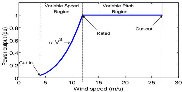
Fig. 1. Wind turbine power curve characteristics [2]
