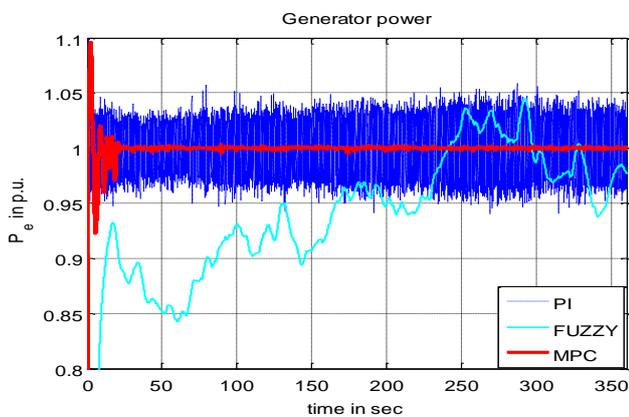
**Fig. 22.** Comparison of generator output power response for simulated wind speed
