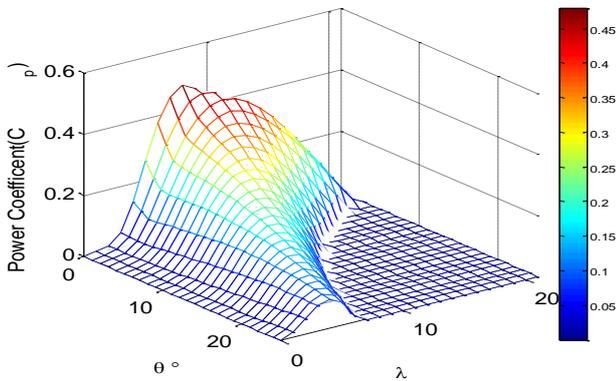
Fig. 3. The power coefficient  $C_p$  as a function of  $\lambda$  and  $\theta$
