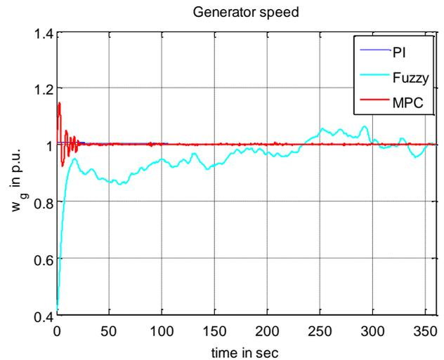
**Fig. 19.** Comparison of generator speed response for simulated wind Speed
