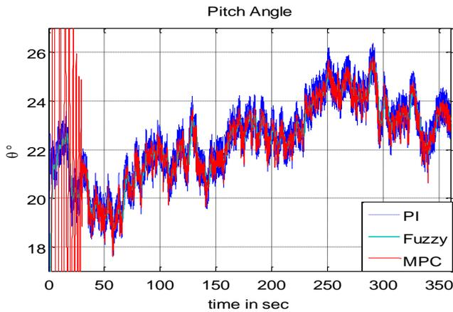
**Fig. 21.** Comparison of pitch angle response for simulated wind speed
