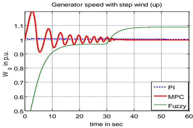
Fig. 9. Generator speed with step wind (Up)
