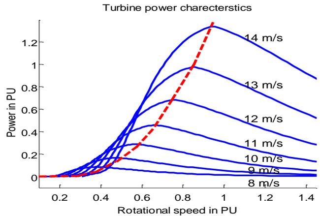
Fig. 5. Turbine Power Characteristics with variable speed
