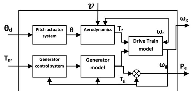
Fig. 2. Control block diagram of WECS [22]
