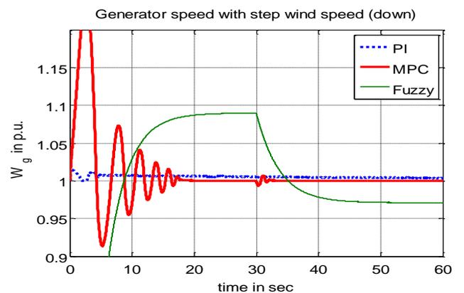
Fig. 14. Generator speed with step wind (Down)
