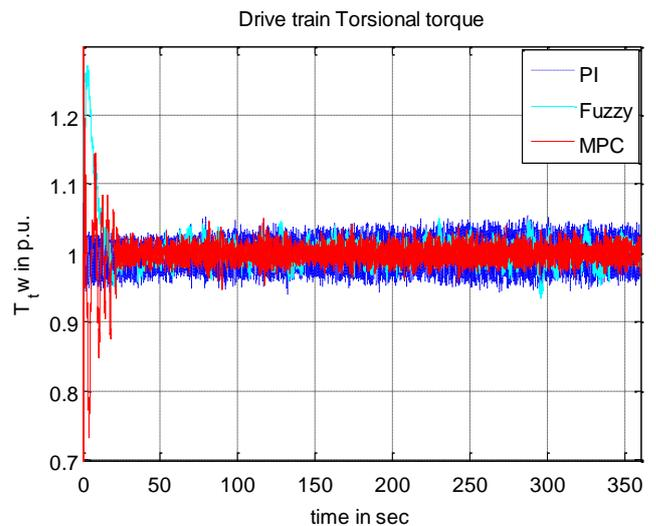
**Fig. 20.** Comparison of torsional torque response for simulated wind speed
