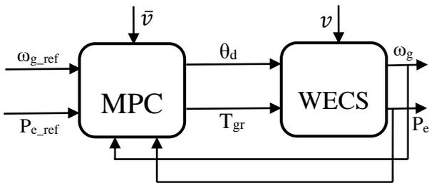
Fig. 7. MPC used as Controller [22]
