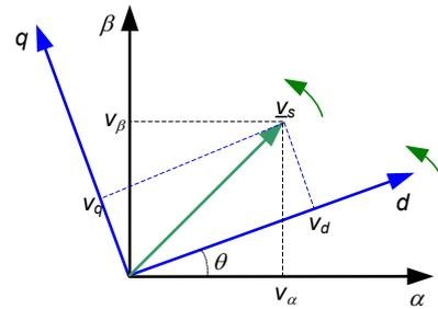
**Fig.2.** Grid voltage synchronization process of the PLL
