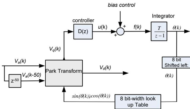
Fig.5. Software dataflow diagram of the designed PLL
