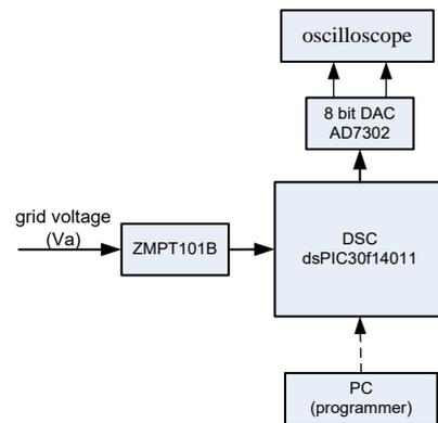
**Fig.3.** Hardware block diagram
