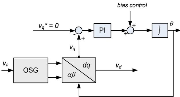
**Fig.1.** Single phase PLL based on orthogonal signal generator
