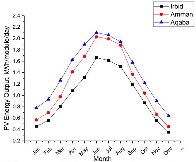
Fig. 7. The average daily PV energy output for one module.
