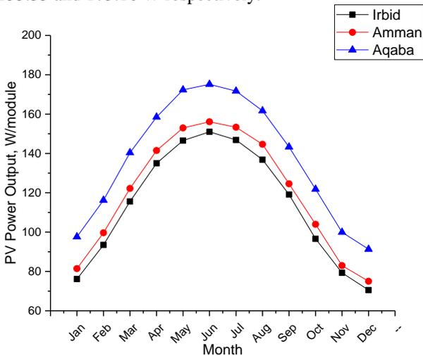
Fig. 6. PV module power output for the three locations
