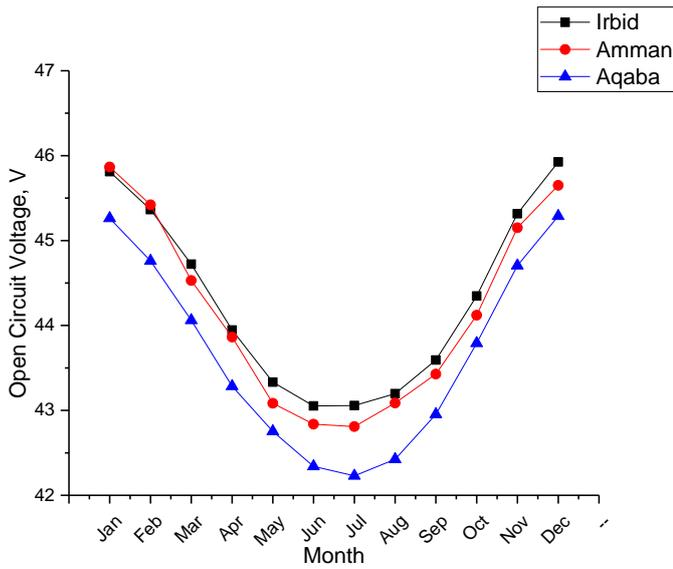
Fig. 5. Average open circuit voltage of PV module for the three locations.
