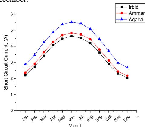
**Fig. 3.** PV module average short circuit current for the three locations.
