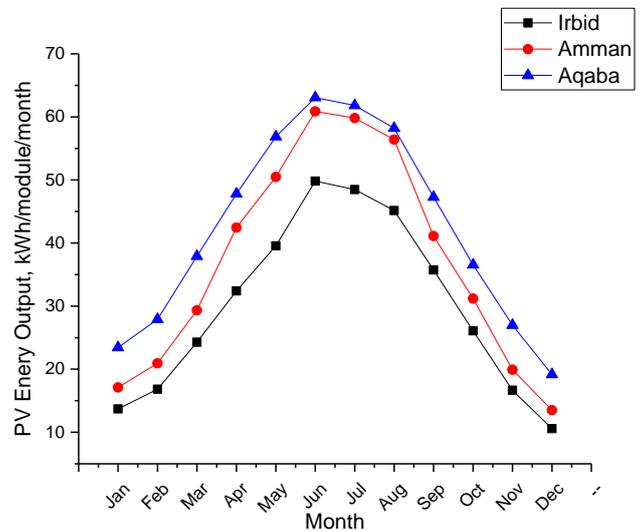
Fig. 8. The monthly PV energy output for one module
