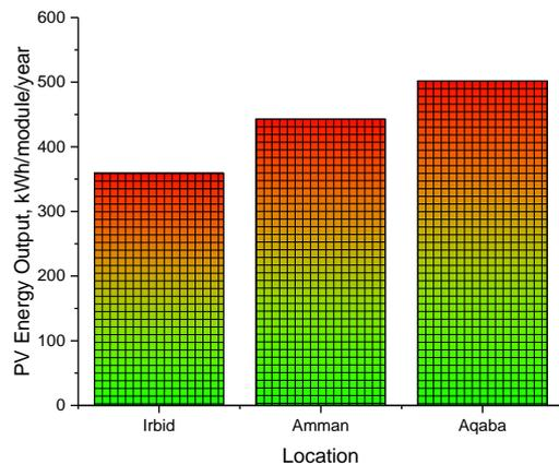
Fig. 9. The annual PV energy output for one module
