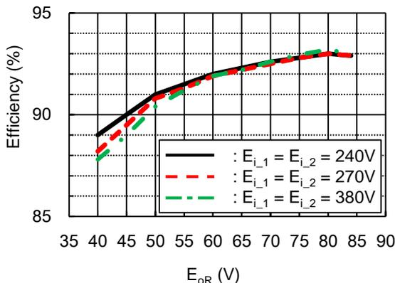
**Fig. 6.** Power efficiency against change of output voltage in parallel operation at  $I_{oR} = 160A$
