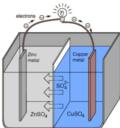
Fig. 7. Electrolysis of copper and zinc metal [67]
