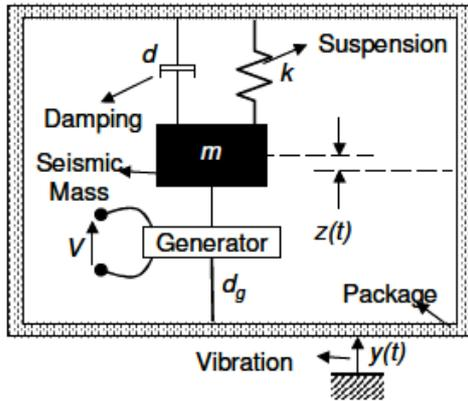
Fig. 1. Schematic overview of vibration harvester [32]
