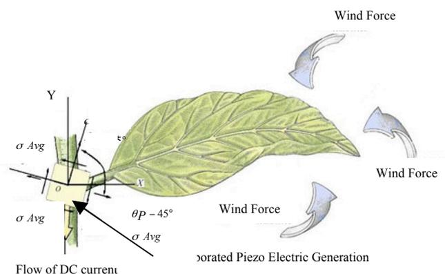
Fig. 3. Piezoelectric harvesting from tree leaf [50]
