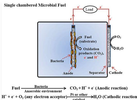
Fig. 8. Principle of single-chambered MFC [75]
