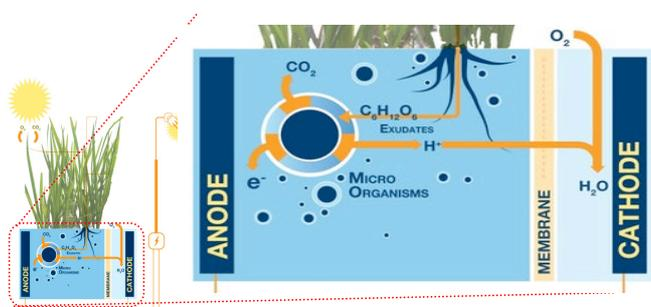
Fig. 9. The reaction of rhizodeposits in P-MFC [80]
