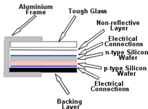
Fig. 5. Construction of photovoltaic cell
